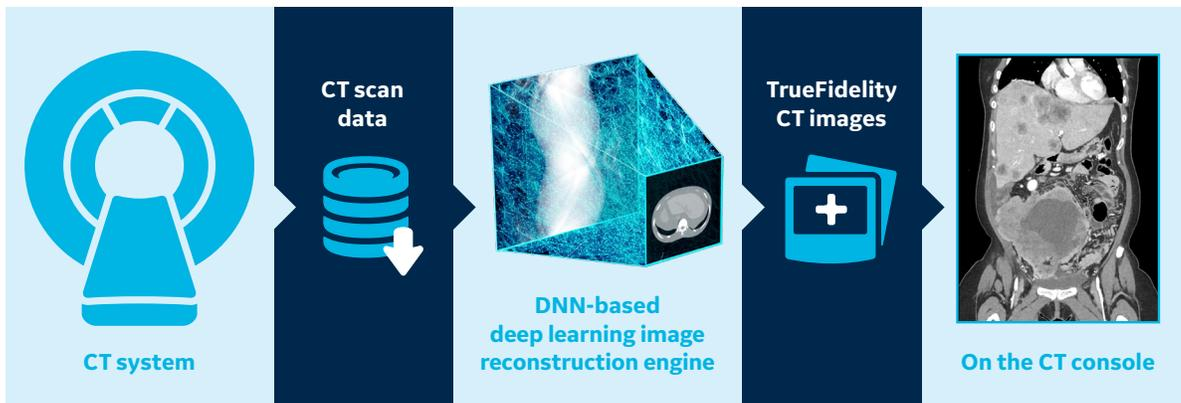
Figure 8: Reconstruction flow of deep learning image reconstruction.
